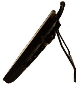
Stand latched in the fully extended position
