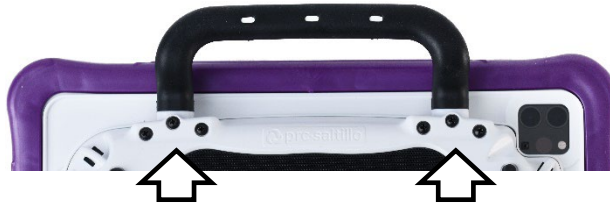
Via Air: Remove six screws
